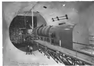
Largest Propeller and Engine Test Cells Completed: Two workers standing inside one of the giant test cells built by Curtiss-Wright for its propeller division are dwarfed by the huge 31-foot stretch which controls air flow in the soundproofed cells and the huge steel tube which regulates correct propeller testing, regardless of engine size. Other photo, taken from inside the true venturi, shows a test cell under operating use of the propellers mounted on a radial engine prior to performance testing. Note interior lighting, soundproof construction and engineer's observation post at upper left.
